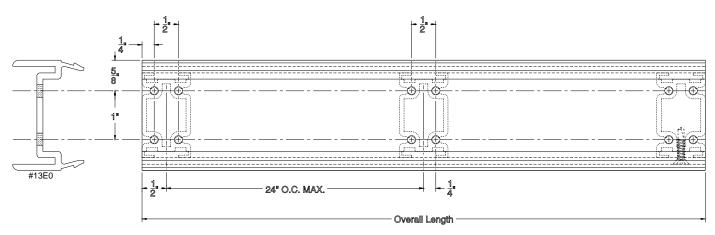
**B.)** Align the holes in the terminator channel with the races in the end of the strut, and attach with the lead-point screws. After all screws have been started, go back and tighten all screws firmly.
