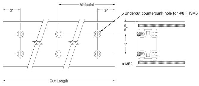
**Note:** Any "raw or sharp" aluminum edges should be smoothed with a file or emery cloth and touch-up paint applied. EFCO provides air dry touch-up paint in any of the standard colors. For custom air dry touch-up paint, contact your local representative for availability and pricing. Any exposed flat head screws should be filled and painted to minimize their exposure.
