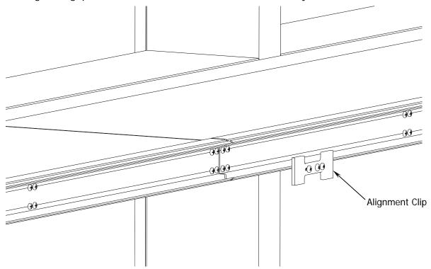
**B.)** Attach the clip with the Tek screws supplied. One (1) screw for each of the fixed holes first and one (1) screw in the approximate center of the adjacent slotted hole into the next light shelf module. It is expected that some minor alignment / adjustments will be needed before the clip is firmly seated, and then the screws are tightened.
