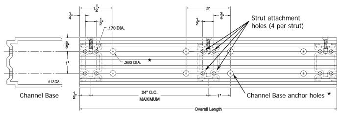
**B.)** Attach all struts with the lead-point attachment screws through the channel base into the strut and tighten firmly.
