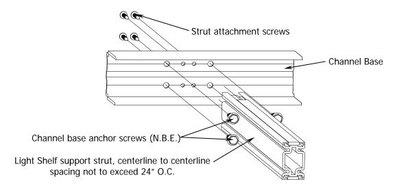
**C.)** Attach the channel base support / strut assembly to the glazed wall product or substrate with \*appropriate size and quantity of fasteners. (\*Attachment fasteners are only sized and provided by EFCO when attachment is to EFCO material.)
