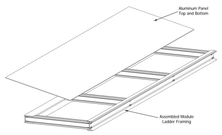
2.) Square the E-Lite Module Ladder to the Panels and Pin.
