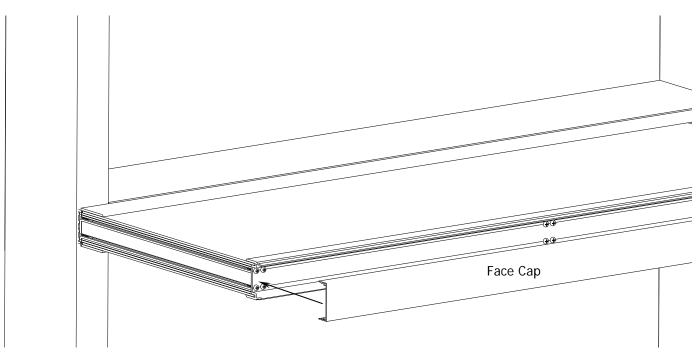
**B.)** Engage the face cap on the upper snap and rotate onto the lower snap. It may be necessary to use a block of wood and a mallet.
